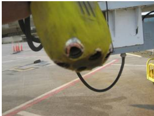
GPU plug end damaged by dragging across the ramp
